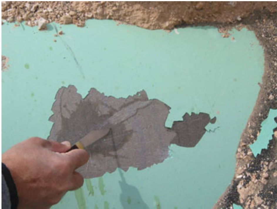
Figure 3-18: Cathodic Blistering/Disbondment of Protective Coating
