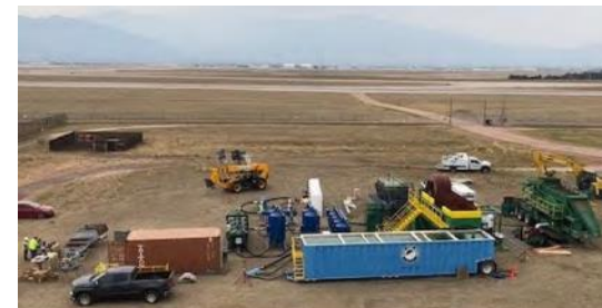
Above: Soil washing system setup
