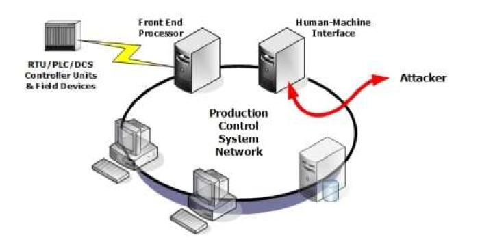
An effective attack is to export the screen of the operator's HMI console back to the attacker (see Figure 14). Off-the-shelf tools can perform this function in both Microsoft Windows and Unix environments. **The operator will see a "voodoo mouse" clicking around on the screen unless the attacker blanks the screen.** The attacker is also limited to the commands allowed for the currently logged-in operator. For instance, he probably could not change the phase tap on a transformer.
