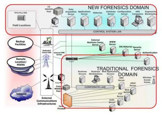
Figure 1. Control systems forensics domain and CSSP reference architecture.<sup>e</sup>
