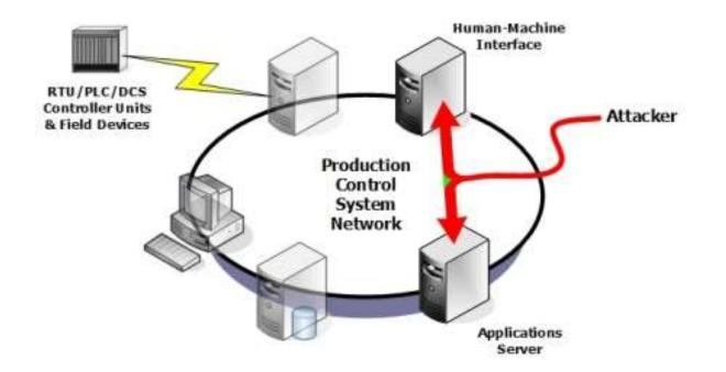
Man-in-the-middle attacks can be performed on control system protocols if the attacker knows the protocol he is manipulating. An attacker can modify packets in transit, providing both a full spoof of the operator HMI displays and full control of the control system (see Figure 16). By inserting commands into the command stream the attacker can issue arbitrary or targeted commands. By modifying replies, the operator can be presented with a modified picture of the process.
