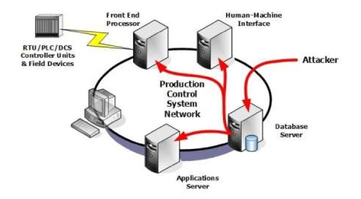
In some, but not all, vendor's control systems, manipulating the data in the database can perform arbitrary actions on the control system
