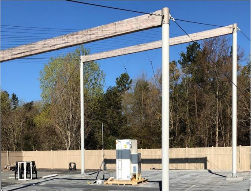
Left: EMP hardened module being tested at EPRI's EMP test facility in Charlotte, NC; Right: 3D E/M simulation of module
