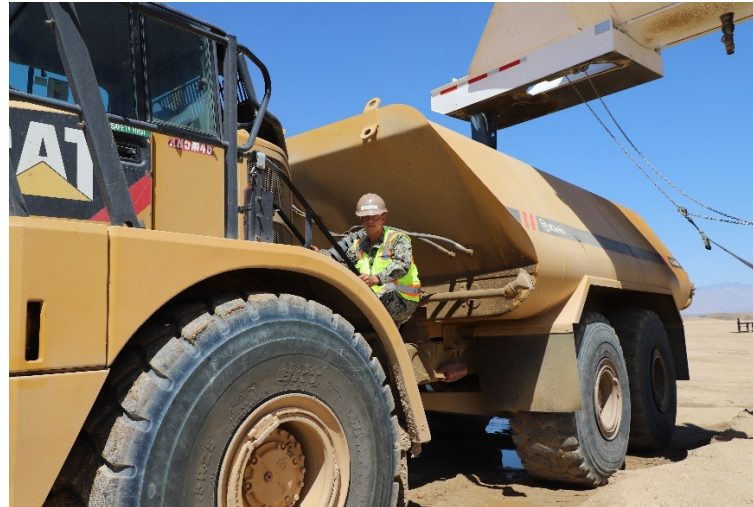
Seabee remounts 8K CAT off-road water truck for dust suppression and soil conditioning on the 158 acre site
