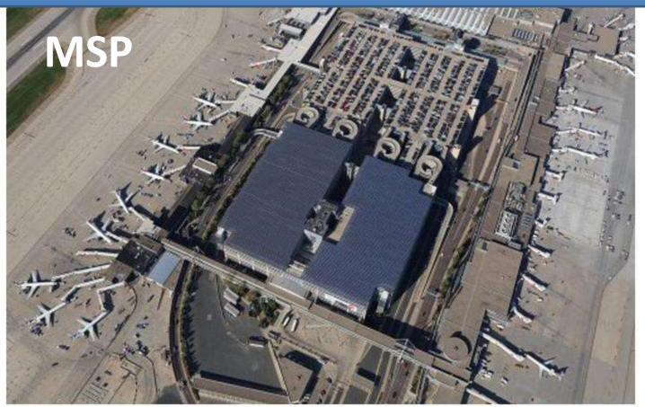
AMERESCO completed a 3-MW project on the top deck of two parking structures at Minneapolis-St. Paul International Airport in late 2015, making it Minnesota's largest solar generation site. In addition to solar, the project converted more than 7,700 light fixtures to LED technology and brought the total number of electric vehicle charging stations to 18. (Credit; Ameresco)
