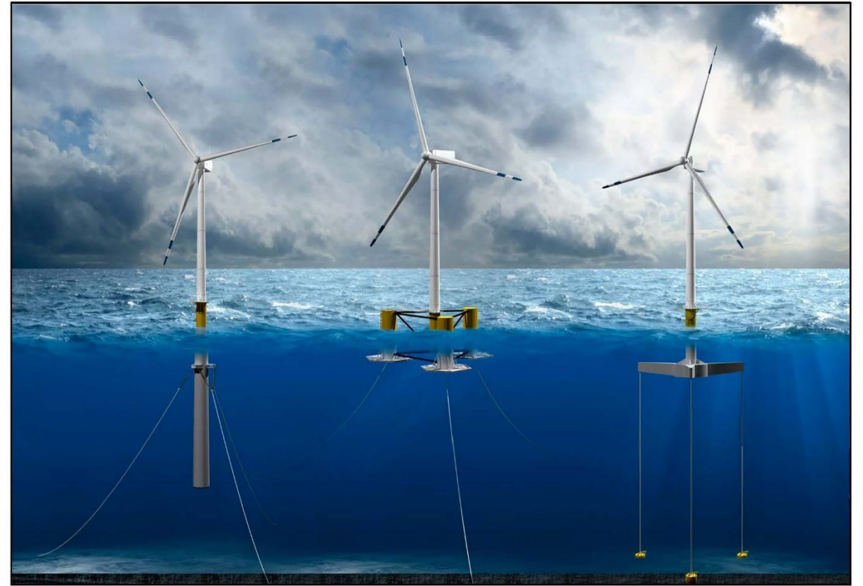
Figure 3.2. Illustration of floating foundation types (left to right: spar, semi-submersible, TLP) (NREL 2022)
