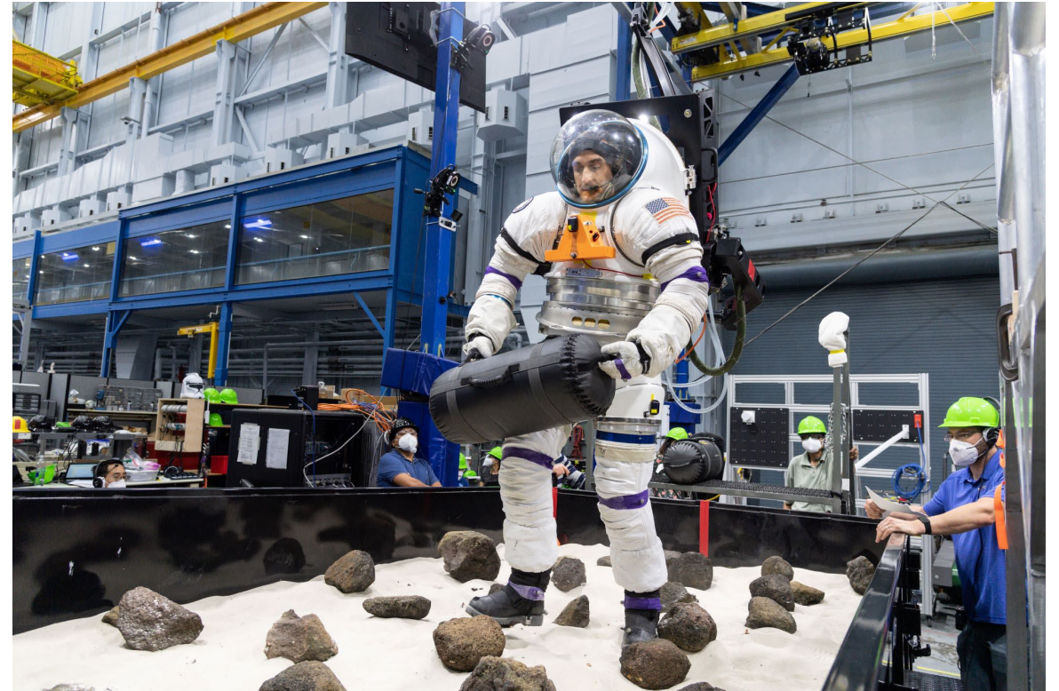
Testing in Active Response Gravity Offload System (ARGOS)
